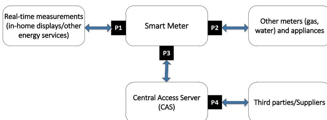
Figure 4.2: Smart meters communication interfaces in the Netherlands.
